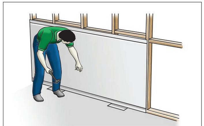
FIGURE 4 FIXING FIRST SHEET
