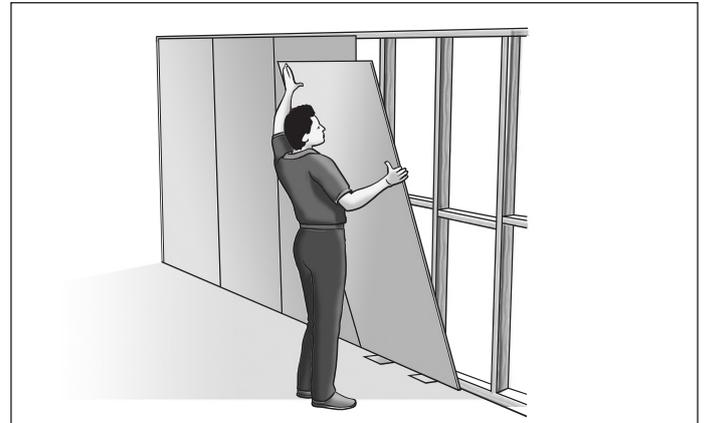
FIGURE 4 SHEET INSTALLATION
