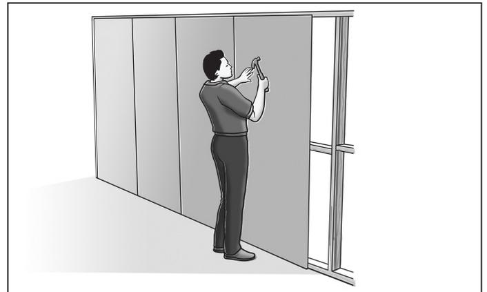
FIGURE 5 SHEET INSTALLATION
